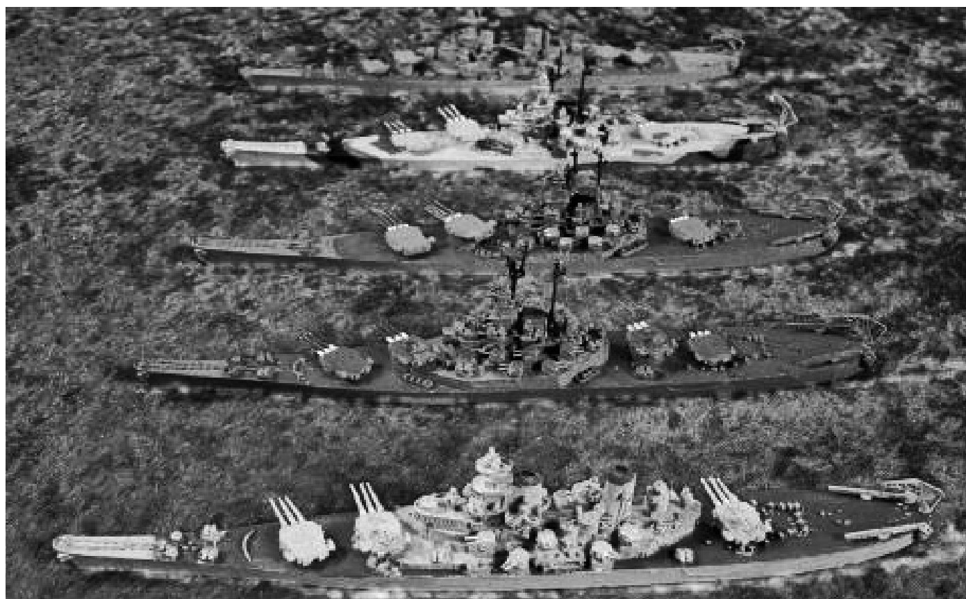
Design variants of the IOWA class U.S. BB's; Front to back: A105 IOWA (Final Design); A132 Design BB65A, A133 Design BB65I, A136 Design BB65C, B205 Design CA2D; Photo and model painting by Bob Weymouth • Note: Photos of the Superior "Never-weres" can be found on our website.
