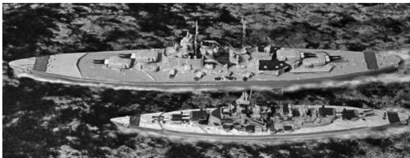
The proposed monster "Never-was" G105 German 128,930 ton, 1200 foot long Battleship Design H44 with its 9-20" guns steams next to the German Battleship G101 BIS-MARCK which was the largest that the Germans actually built displacing 41,700 tons, 792 feet in length and carrying an 8-15" main battery.
